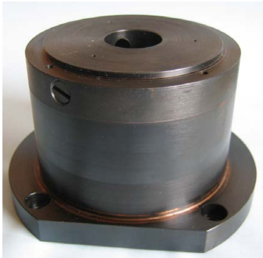
Steel brazed with copper
