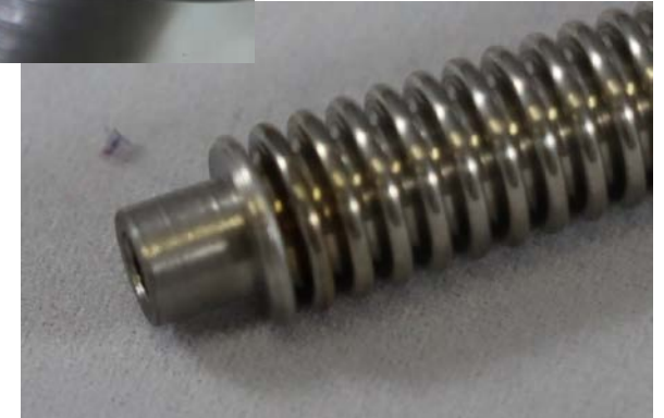
bellow – flange 0.3 mm thick, \varnothing 10 mm
