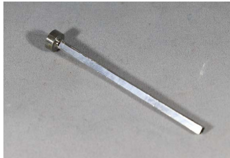
Iridium square tube, 2x2 mm, 0.2 mm thick
