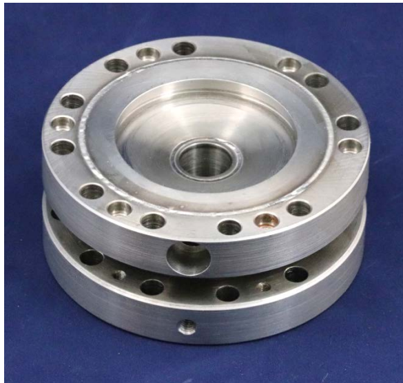
Stator body, 8 welds
