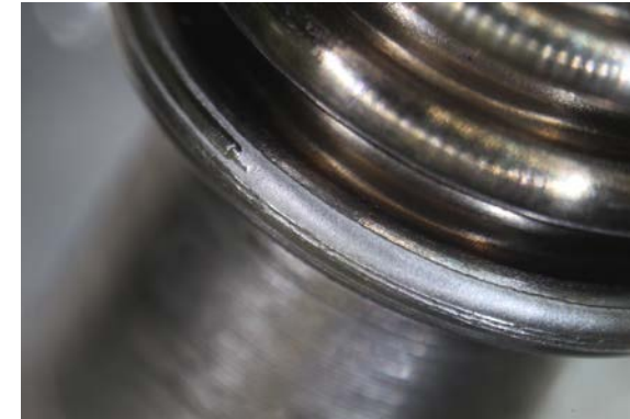
bellow – flange 0.3 mm thick, \varnothing 10 mm
