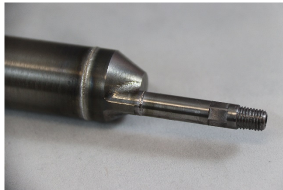
Tantalum target Ø30 mm, Ø8 mm
