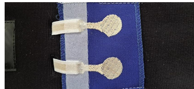
Embroidered textile electrodes hot-bar welded to a conductive elastic ribbon for EMG monitoring
